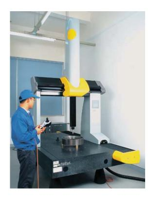
Surveying machine with three coordinates
