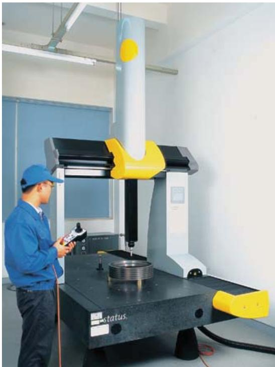
Surveying machine with three coordinates
