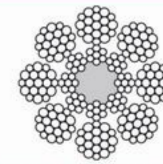
Construction: 8 x 19 Warrington with steel reinforced core, regular lay Number of load bearing wires: 152 结构: 8x19,带钢制增强芯,瓦林吞式, 交互捻 承载钢丝数量:152
